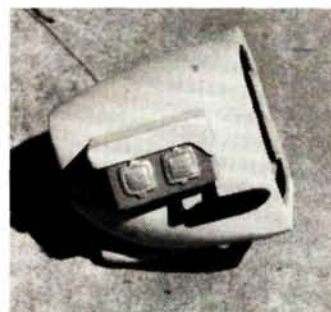
Nose cowling block is built-up. Note dummy engine.
