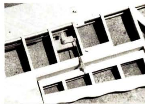
Aileron hookup requires no-slop linkage.
