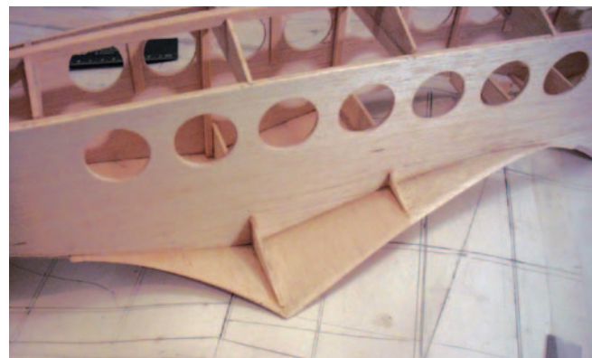
The bottom sheeting forms the base of the wing fillets.
