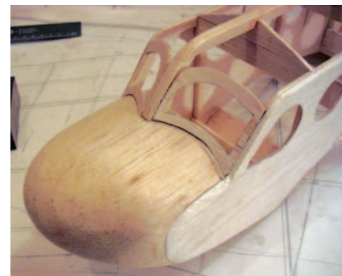
Sand and shape the nose block before you install the windshield frames. The bottom edges will need some beveling to fit. Lightweight spackling fills the gaps.
