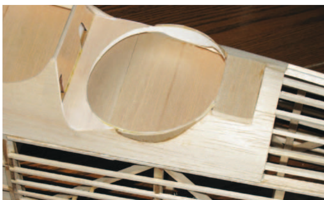
1/16-inch sheeting around the cockpit area, showing the ring-mount detail.
