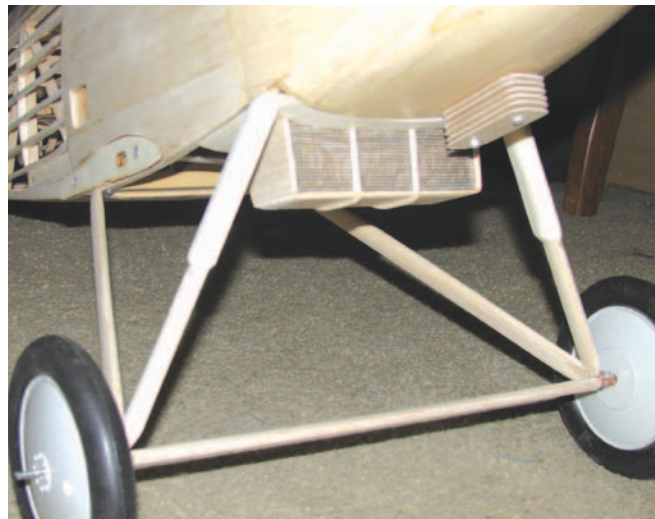
The landing gear is of the conventional soldered-music-wire type, with balsa fairings added. The dummy radiator and cooling fins are built up from scrap balsa and a bit of screen material.
