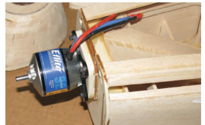
The E-flite brushless motor dry-mounted. The author needed to add an additional 1/4-inch plywood block to bring the propeller collet flush with the nose.
