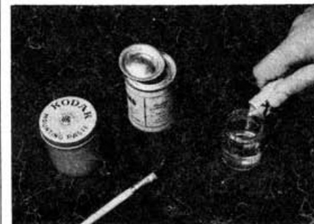
Dope thickened with cement (must be same type), or photo mount paste are suitable adhesives to attach the edges of covering to the framework.
