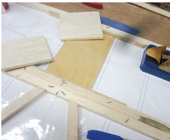
The center of the horizontal stabilizer is a sandwich of balsa and plywood sheeting.
