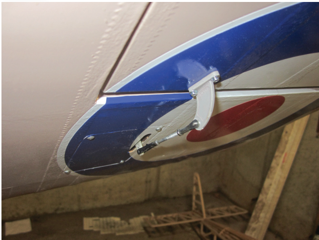
The aileron servos are installed under flush-fitting hatch covers. I used 4-40 hardware for all linkages. I used Robart control horns throughout.
