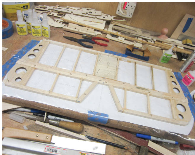
Shown here is the completed stab and elevator assembly.
