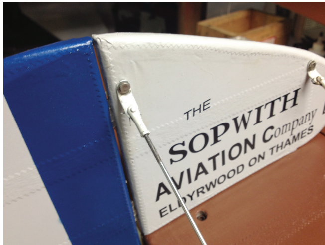
I used miniature clevis ends for the tail-surface rigging wires.
