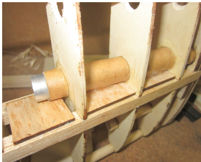
The lower wing panels have the cardboard tubes to mate with the aluminum wing tube that runs through the fuselage.
