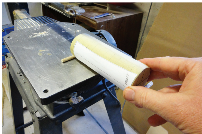
The trickiest piece to make is cut from a 2-inch wood dowel, which will become the top part of the engine cover.
