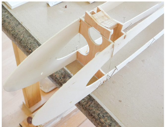
The fuselage structure is also very easy to build. Here some of the formers are glued in place between the two fuselage sides.
