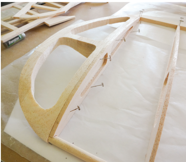
Here's a closeup of the wingtip structure being glued to the outer rib of the wing.
