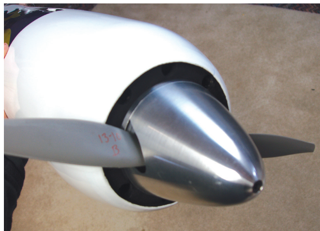
The cowling opening is dominated by the big Tru-Turn spinner.
