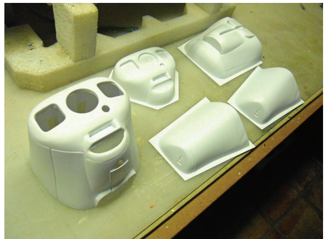
The vacuum-formed engine cowl from Parkflyerplastics.com is easy to assemble from the parts shown here.
