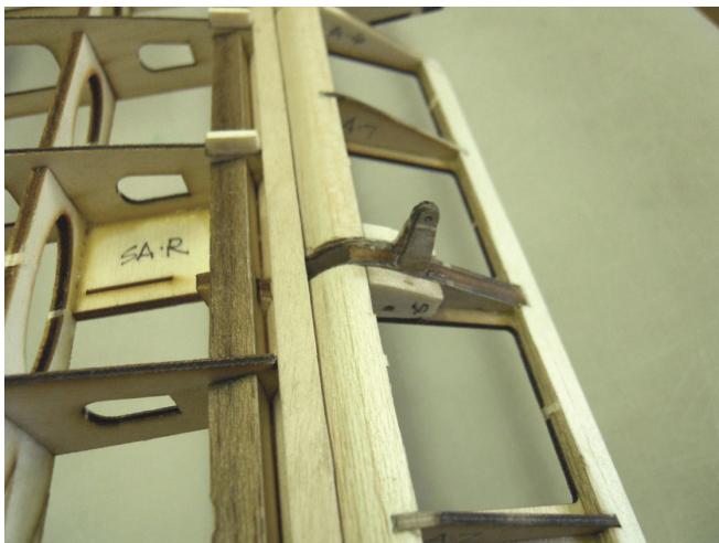
Here you see the scale shape of the flaps. All the parts are shown on the plans, drawn with CAD for accuracy.
