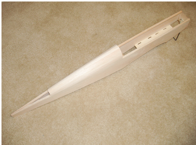
The basic fuselage structure is a simple box arrangement with sheeted aft decking.
