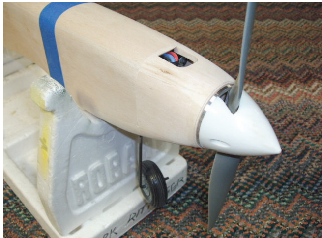
The motor and spinner are faired in with balsa blocks to form the cowl. I use silicone adhesive to hold the cowl in place after it has been shaped and covered.
