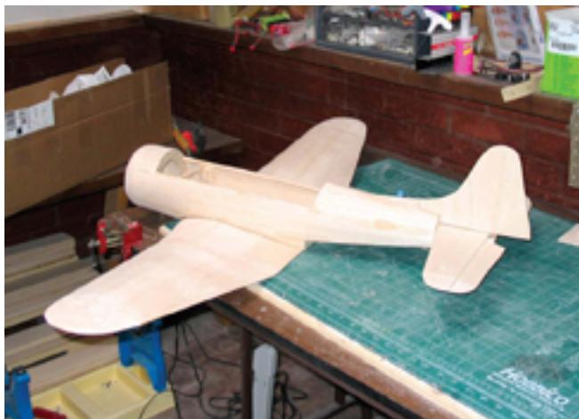
With the wing joined to the fuselage, the airplane begins to resemble a Navy torpedo bomber.
