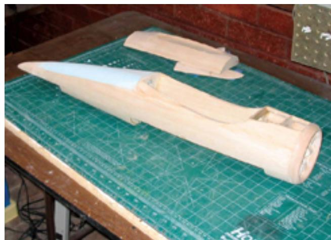
The aft belly section is made out of a foam block, carved and sanded to shape.
