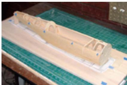
Here is the fuselage with its side sheeting in place.
