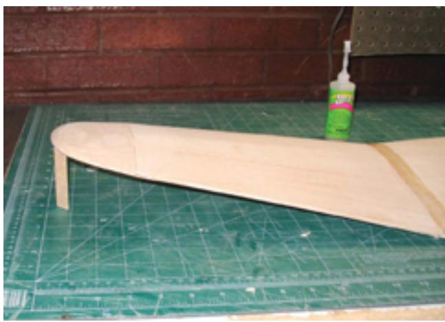
When you glue the outer wing panels to the center section, block up the tip to the proper dihedral angle and then wrap the panel joints with fiberglass tape and glue for strength.
