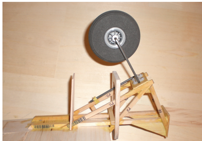
The landing gear assembly is sturdy and easy to build. The gear is designed to absorb rough field shocks and bumps.
