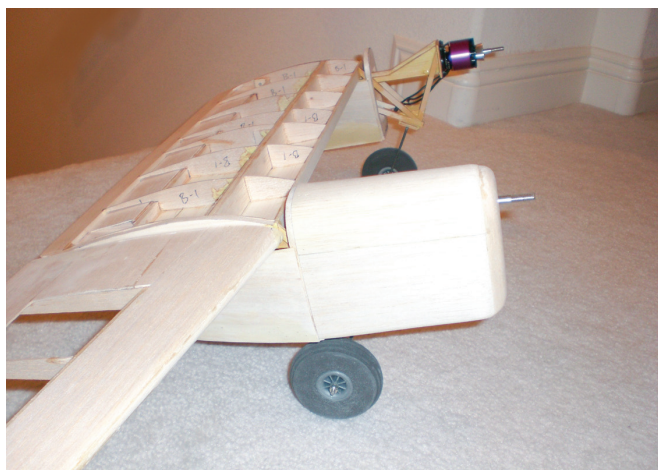
One of the engine nacelles has been sheeted and sanded to shape.
