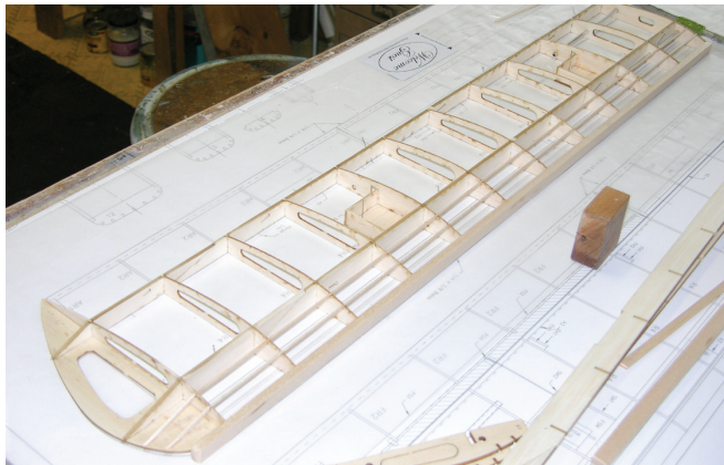
The wing is built up in an eggcrate fashion with the ribs slotted onto the main and rear spars. The servo mounts and other internal components are added after the main assembly is complete.
