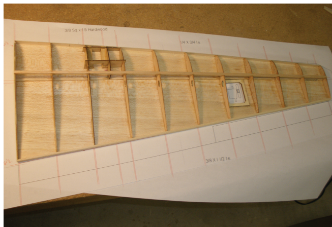
Right wing completed. Need to cut holes for retract assembly and wheel opening before adding top sheeting. Don't forget to add pull strings for retract and aileron wiring.
